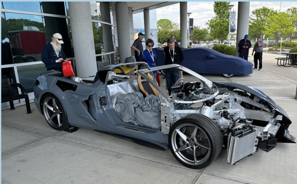
Cutaway of the E-Ray, front motor, and rear engine.
